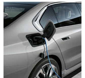
The fast charging cable (mode 3) allows you to charge the high-voltage battery at public charging stations – 3-phase and with a charging capacity of up to 11kW.
